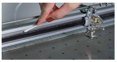
the bottom side of the rail. You will need to move the X-axis belt out of the way to access the rail. There is enough flex in the belt to move it out of the way, but do not pull on it so hard that it becomes stretched or stressed.
